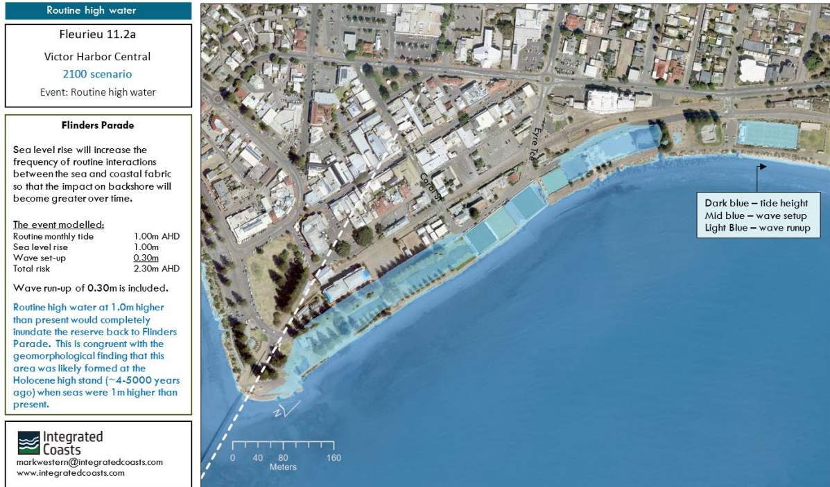
Figure 30: Modelling for 2100 scenario for routine highwater events for Flinders Parade. These routine events are expected to occur a few times month from April to September (M. Western).
