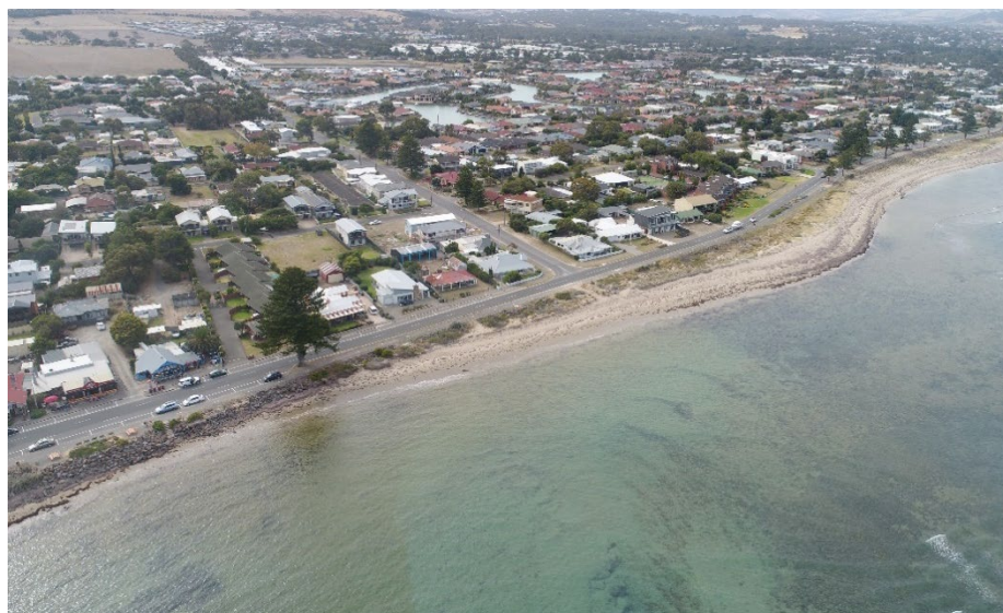
Figure b. The area between Yilki and Tabernacle Road were likely nourished and vegetated by Council in the 1980s. (The only other explanation is that this area accreted and was vegetated but this is unlikely given the timing of the Council's works.)
