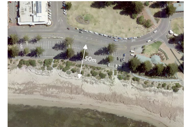
Figure b: Legacy issues- the carpark constructed ~20m from the highwater mark and storm water outlets that prevent a stable dune system from being established on the beach.
