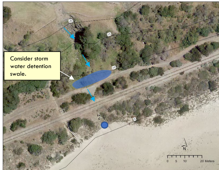
Figure a: Storm water outlet currently drains directly on to the beach and prevents the dune from forming in this location. Recommendation to extend the outlet pipe and form the dune to the main vegetation line but using construction methods that can reduce the length of the pipe in the future if the coast goes into an erosion cycle.
